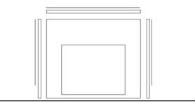
Step #5 Install mounting strips 1/2" or 3/4" Inside of lines
